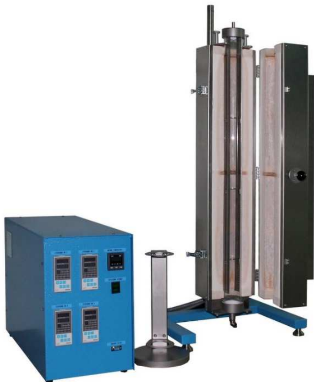
Figure 18. Split tubular furnace on stand used for plastic scintillator cylinders synthesis [151]
