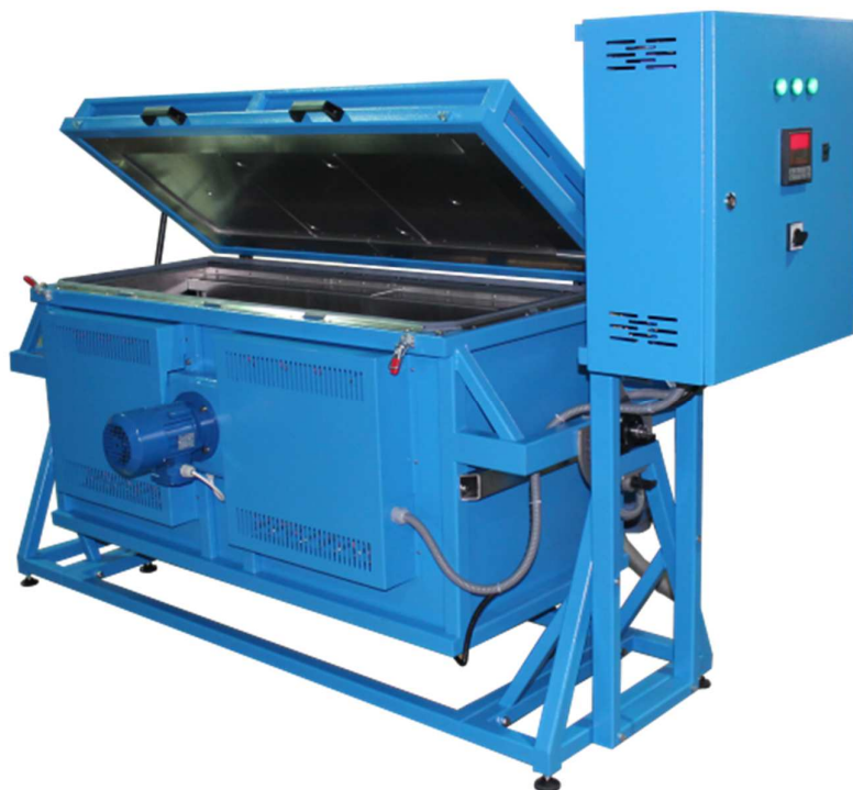
Figure 22. Furnace for plastic scintillator plates manufacturing [157]
