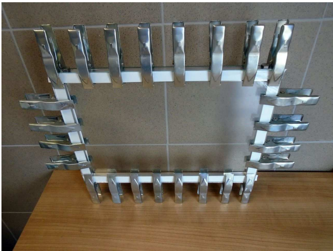
Figure 21. Photograph of mold consisting two 280x400 mm glass plates, aluminum frame, white teflon gasket and steel spring clamps.
