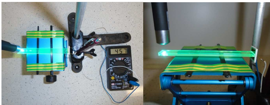
Figure 39. Photograph of experimental setup used in measurement for wavelength shifter bars: top view (left) and side view (right)
