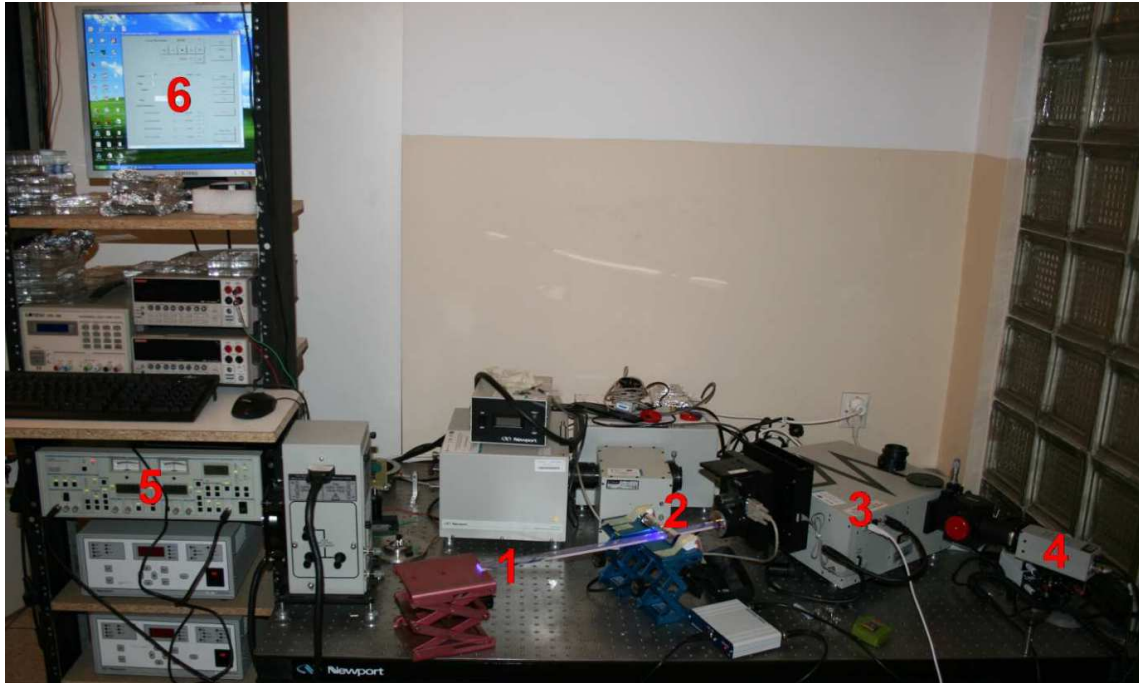
Figure 44. Scheme (upper panel) and photo (lower panel) of the experimental setup used in measurement of emission spectra of 5x19x500 mm 3 EJ-230 plastic scintillator strip. UV lamp exciting scintillator was moved along the scintillator strip. Numbers on lower panel photo denote 1 scintillator, 2 UV lamp, 3 monochromator, 4 detector, 5 lock-in amplifier, 6 PC to control the monochromator [175].
